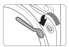
1. Loosen all shipping bolts on the rear of the machine using the supplied spanner.
