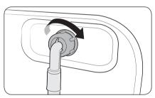
Connect the other end of the water hose to the inlet valve on the back of the washing machine, and then turn it to the right to tighten.
