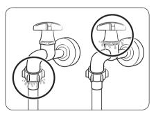
Slowly open the water tap and check if there are any leaks around the connection areas. If there are water leaks, repeat step 1 and 2.
