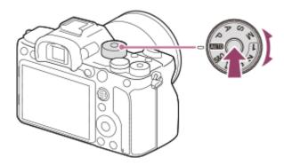
Turn the mode dial while pressing the mode dial lock release button in the center of the mode dial.
