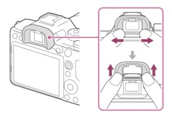
Remove the eyepiece cup when attaching an angle viewfinder (sold separately). Also, select MENU  $\rightarrow$  (Camera Settings2)  $\rightarrow$  [FINDER/MONITOR], and then switch [Viewfinder(Manual)] and [Monitor(Manual)].
