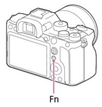
2 Select the desired function by pressing the top/bottom/left/right side of the control wheel.
