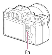
Select the desired function by pressing the top/bottom/left/right side of the control wheel.
