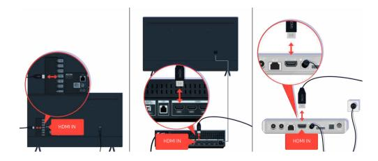
Check the antenna and HDMI cable connections.
