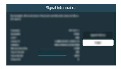
Signal strength must be more than 20 dB (more than 4 bars on the icon) for stable signal reception.
