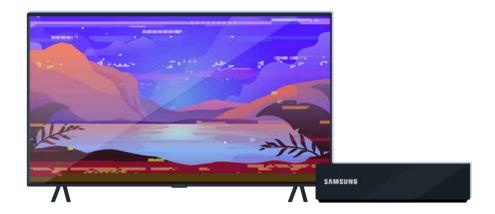
Check the antenna and input cable connections.
