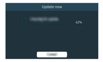
The firmware update begins automatically. Your TV will automatically reset when the firmware update is completed. Do not turn off your TV while the firmware update is in progress.
