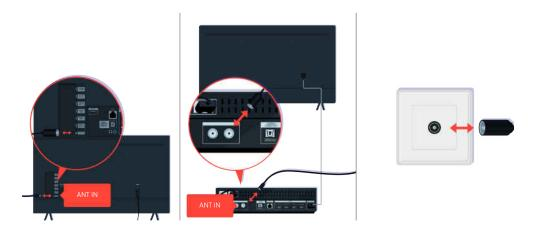
Check the antenna and input cable connections.
