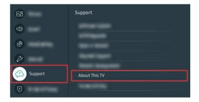
Select (a) > (3) Settings > Support > About This TV and check the model code and software version.
