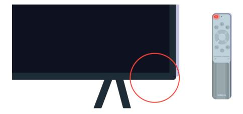
If the remote control sensor turns off when you press the power button, your TV is correctly connected to the power supply.
