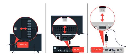
First disconnect and reconnect the power cables and HDMI cables on the back of your TV or the One Connect (OC) Box, then unplug the power cord and plug it back into the wall outlet.
