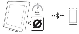
1. Press (Mic On/Off) button for 3 seconds for pairing.
