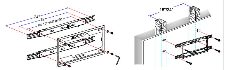
Solution 3. If studs spacing is over 16"(less than 24") or not in your desired position, apply 24" extension plate MD5232 (available on Amazon.com) to bridge up wood studs up to 24".
