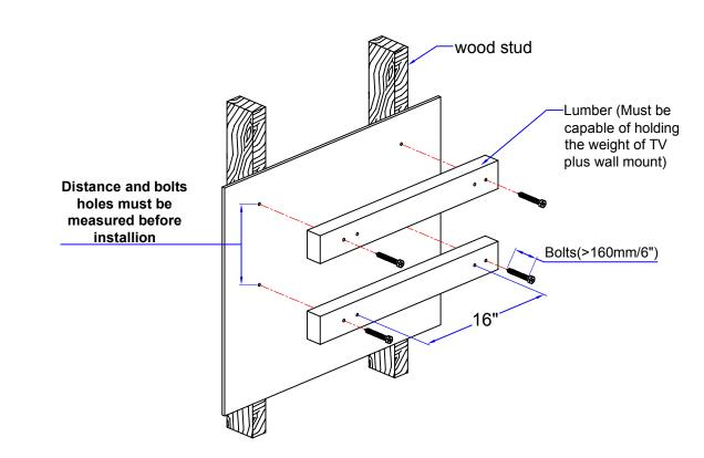
Step 2 Please locate your 16" wall plate at the position you desire then use bolts and washers (both provided in hardware bag) to attach 16" wall plate to installed lumber.
